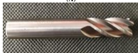
Fig. 4: (A) Parallel shank 4F Endmill with designated dimensions [15], (B) Cutting tool used for experimental runs.
