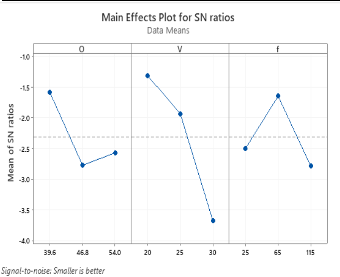
Fig. 7: Effects of overhanging of tool, cutting speed and feed rate on S/N ratio.
